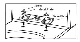
5. Install the bidet: push the cover backward as shown in the figure (as shown in the figure below).
