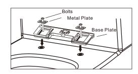
5. Install the bidet: push the cover backward as shown in the figure (as shown in the figure below).
