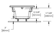
Wood support design may vary. All dimensions are approximate. Structure measurements must be verified against the unit to ensure proper fit.
