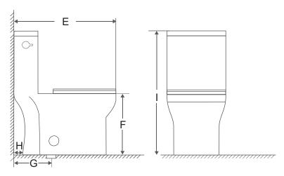
A.380mm(14-61/64") B.150mm(5-29/32") C.470mm(18-1/2") D.370mm(14-9/16") E.690mm(27-11/64") F.400mm(15-3/4") G.300mm(11-13/16") H.65mm(2-9/16") I.765mm(30-1/8")
